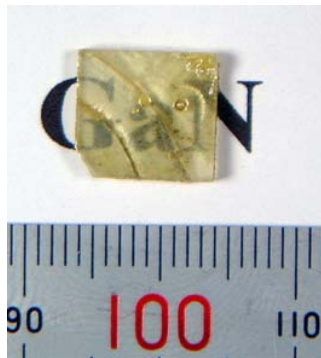
Fig. 14. A transparent GaN crystal as grown by the acidic ammonothermal technique.
